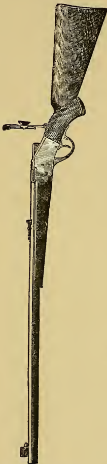
Fig. 102.—Sharps-Borchardt Off-Hand Target Rifle.
